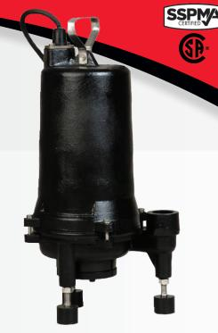
2 HP grinder pumps that have a 1 1/4" vertical discharge (optional 2" adapter available), and can grind up to 3" solids, and be installed on a rail system or with the supplied legs
