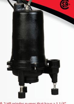
1 & 2 HP grinder pumps that have a 1 1/4" vertical discharge (optional 2" adapter available), and can grind up to 3" solids, and be installed on a rail system or with the supplied legs
